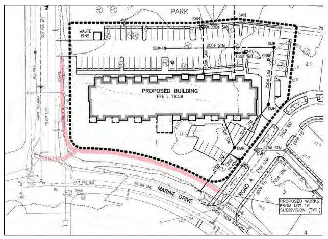
Figure 2: Sidewalk and Crosswalk Mark-up
